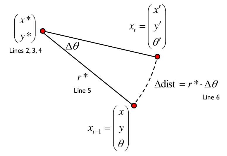
• given  $\Delta \theta$  and  $\Delta dist$  we can compute the velocities needed to generate the motion
